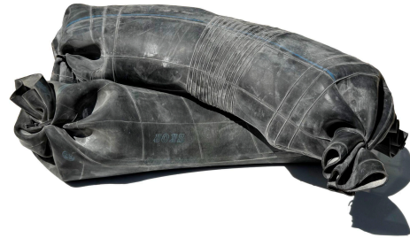
Sandbags. These are flexible supports that will cushion and hold your stone at different angles for carving. They are made from tractor tire tubes, sand, and zip ties.
